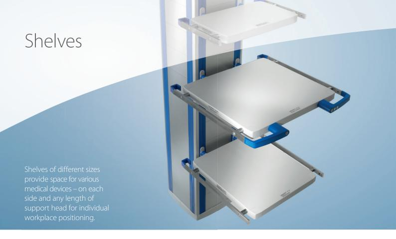
For the TruPort<sup>m</sup> Supply Unit we offer shelves in five heavy load versions (HL - 80 kg / 176 lbs) and two medium load versions (ML - 50 kg / 110 lbs) of various sizes. The shelves can be mounted to the system head without tools by means of the click mechanism.
