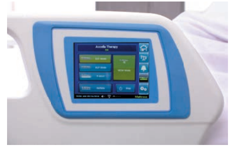
Surface controlled through the Graphical Caregiver Interface on the Hill-Rom 900 Accella Bed
